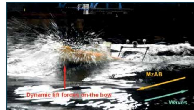
Figure 2: MzAB in head waves (180°), boat speed 8.5 kn, wave length 10 m, wave height 1.0 m
