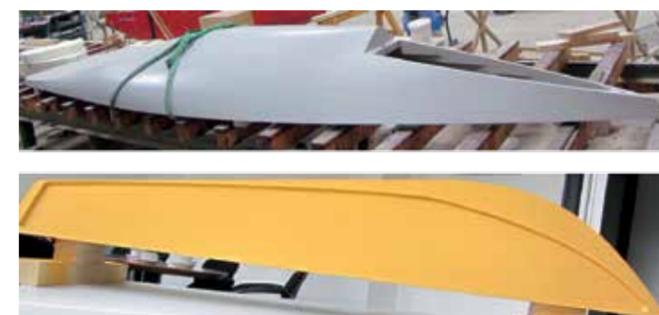
Figure 3: Water-tunnel test model: Main body (top) and interchangeable bow segment (bottom)
