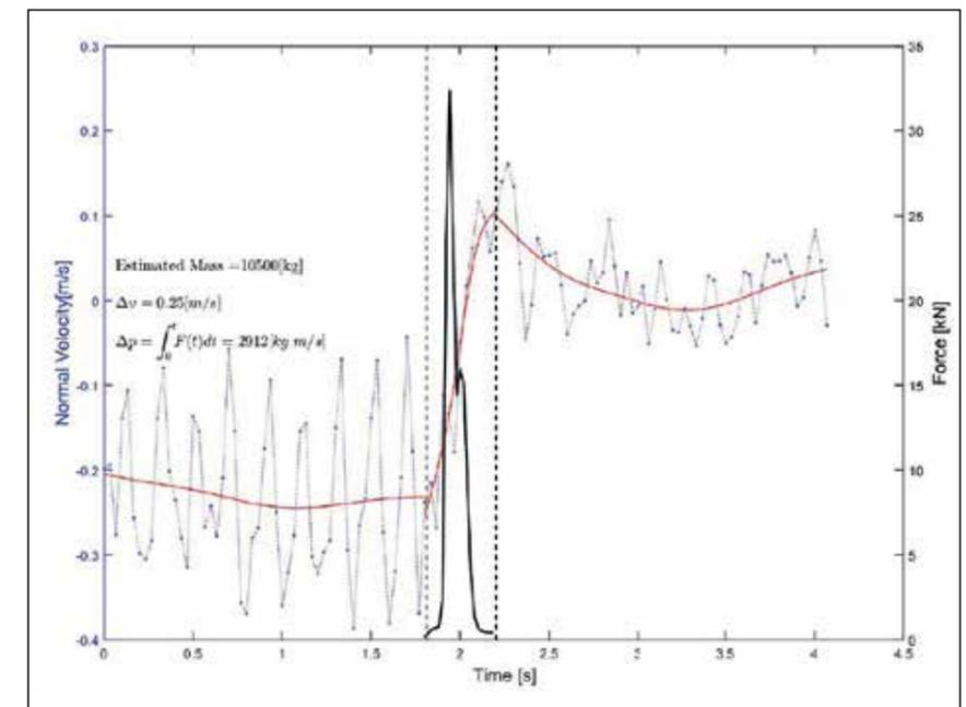
Figure 9: Momentum Analysis of Ice Ship Interaction
