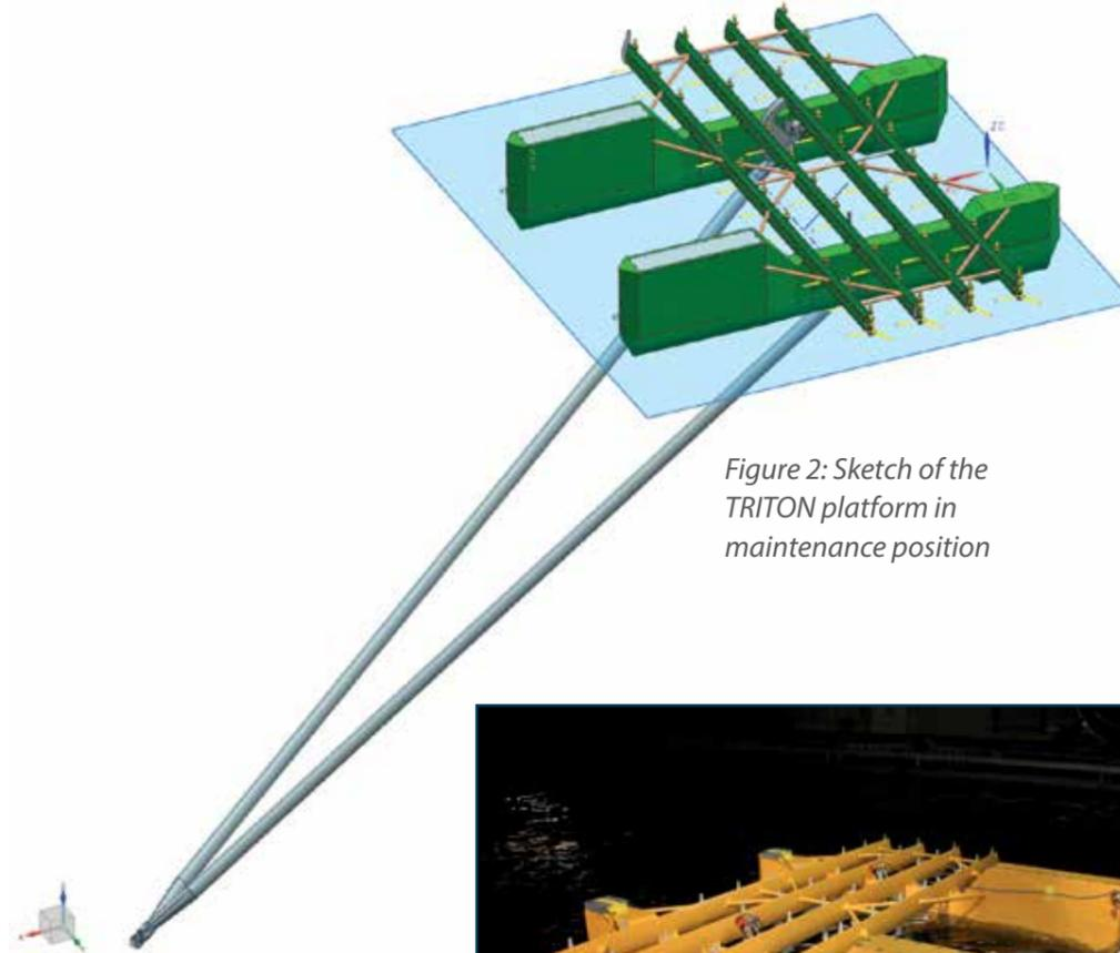
Figure 2: Sketch of the TRITON platform in maintenance position
