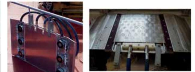
Figures 3 and 4: New Magnetic Ice Force Panel Sensor
