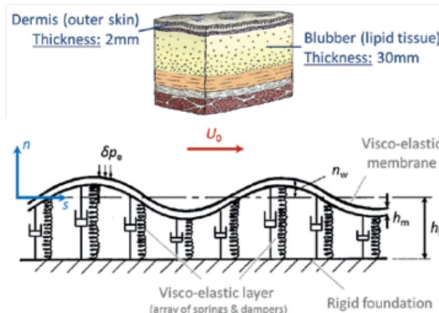
Figure 4: Dolphin skin: Cross section (top) and mechanical model (bottom)
