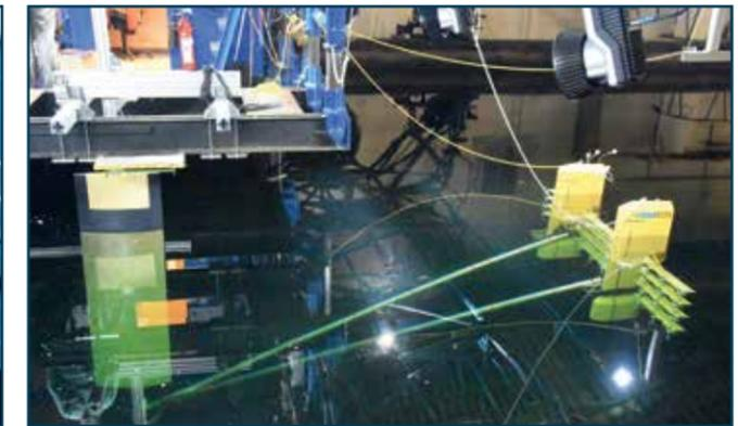
Figure 3: Fully equipped TRITON model in the maintenance mode (left) and test setup with the platform in operating position (right)
