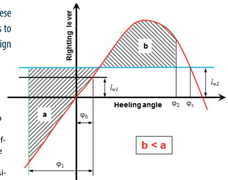
Figure 1: Conventional Weather Criterion
