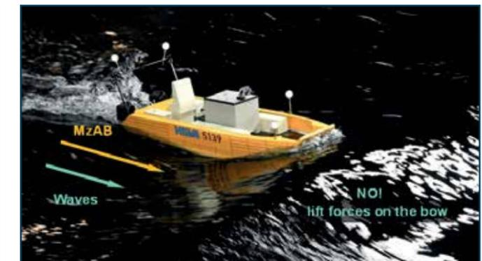
Figure 3: MzAB overtaking following waves (0°), boat speed 8.5 kn, wave length 10 m, wave height 0.6 m. At waves higher than 0.5 - 0.6 m instant flooding can occur
