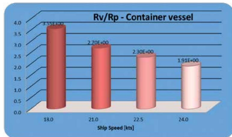
Figure 1: Relation viscous resistance / pressure resistance as a function of speed for a medium sized container ship
