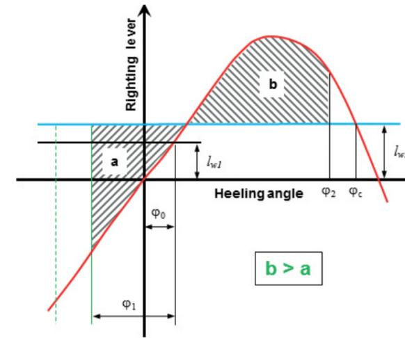
Figure 2: Weather Criterion with decreased angle of roll  $\varphi_1$
