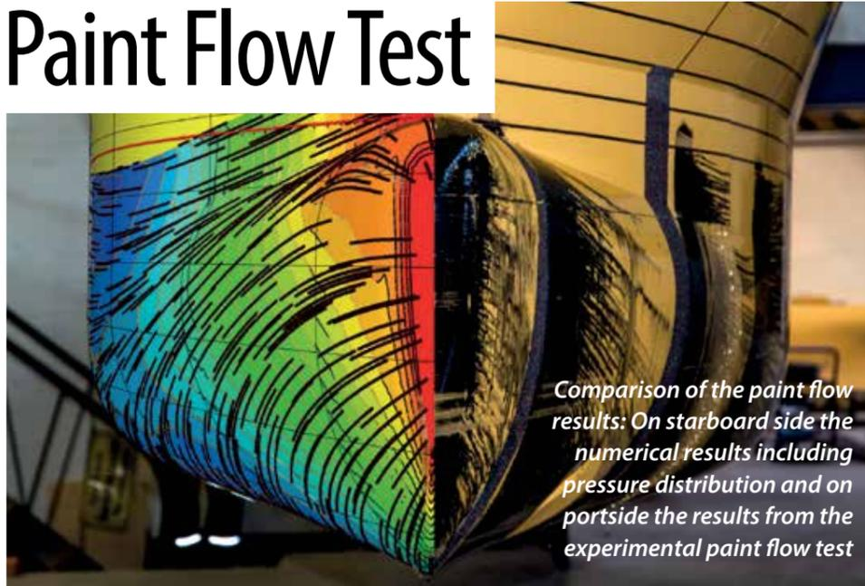
Comparison of the paint flow results: On starboard side the numerical results including pressure distribution and on portside the results from the experimental paint flow test
