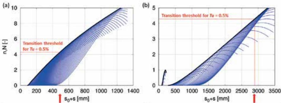
Figure 7: Prediction of the transition point by the  $e^N$  criterion after Mack [7], assuming a turbulence intensity of  $Tu = 0.5\%$  in the test section of the HYKAT water tunnel. (a) Rigid surface: Transition to turbulence occurs approx. 0.5 m downstream of the stem (red arrow). (b) Compliant surface ("blubber": silicone, "dermis": polyethylene): Transition to turbulence occurs approx. 2.9 m downstream of the stem (red arrow)
