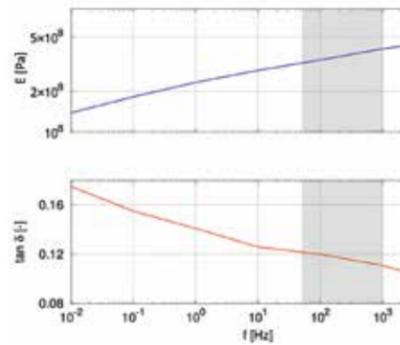
Figure 5: Dynamic mechanical analysis of a thin polyethylene film (data by Fraunhofer-IFAM): Stiffness (E-modulus, top) and damping (loss tangent, bottom) versus excitation frequency. The shaded area marks the frequencies of interest for transition delay
