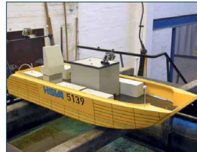
Figure 1: The HSVA Model of the multipurpose workboat MzAB with an IBC-container on deck
