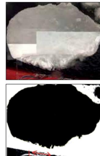
Figures 7 & 8: Stitched Pictures of an Ice Floe (left); Area Analyses of Floe Shape (right)
