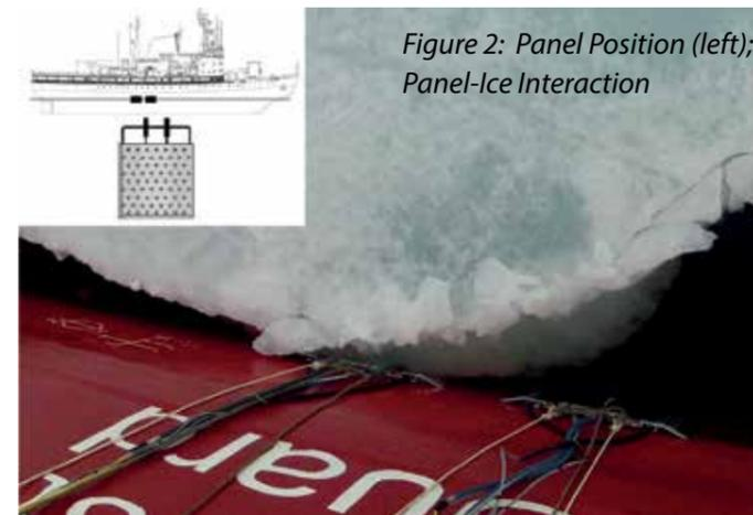
Figure 2: Panel Position (left); Panel-Ice Interaction
