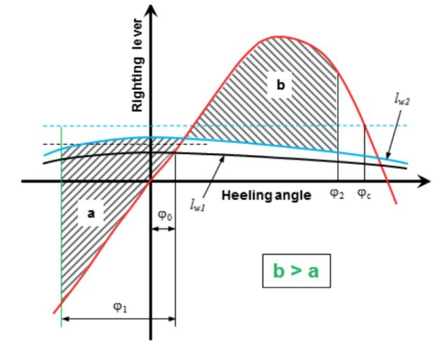
Figure 3: Weather Criterion when the wind heeling lever is reduced and dependent on the heeling angle
