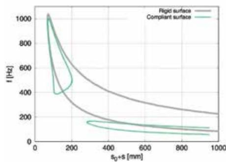
Figure 6: Stability diagram for slightly accelerated Falkner-Skan flow, modelling the laminar boundary layer along the bow of the SAR vessel. The diagram shows regions of amplifying TS waves for a rigid (uncoated) and a compliant (coated) bow surface ("blubber": silicone, "dermis": polyethylene)
