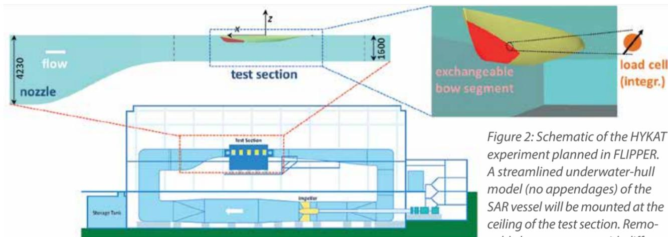
Figure 2: Schematic of the HYKAT experiment planned in FLIPPER. A streamlined underwater-hull model (no appendages) of the SAR vessel will be mounted at the ceiling of the test section. Removable bow segments with different coatings, supported by a load cell, can be inserted into the main body
