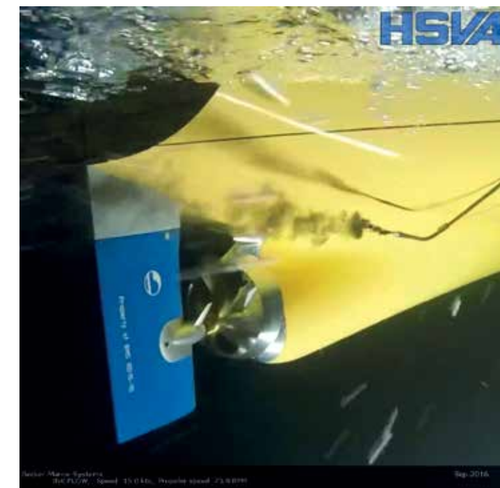
Figure 1: Flow separation at the stern area, detected with the help of an Ink Flow Test
