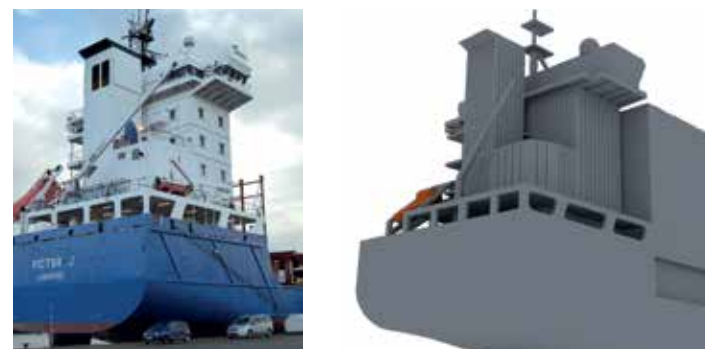
Figures 5 and 6: Planned test ship for full-scale application (left), model for CFD computations (right)
