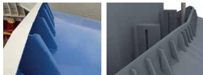
Figures 7 and 8: Details at forecastle shelter: test ship (left), model for CFD computations (right)
