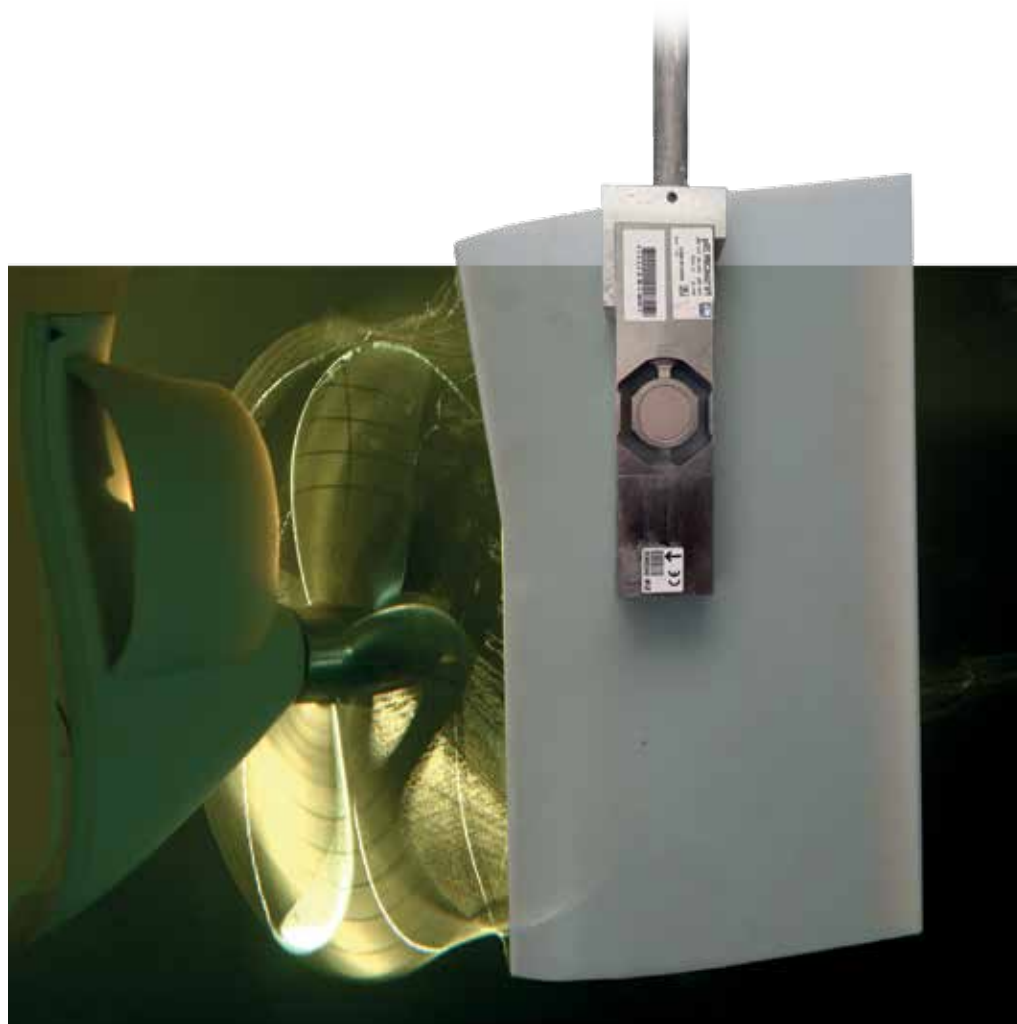
Figure 2: Conventional rudder with load cell in front of the installed rudder during test
