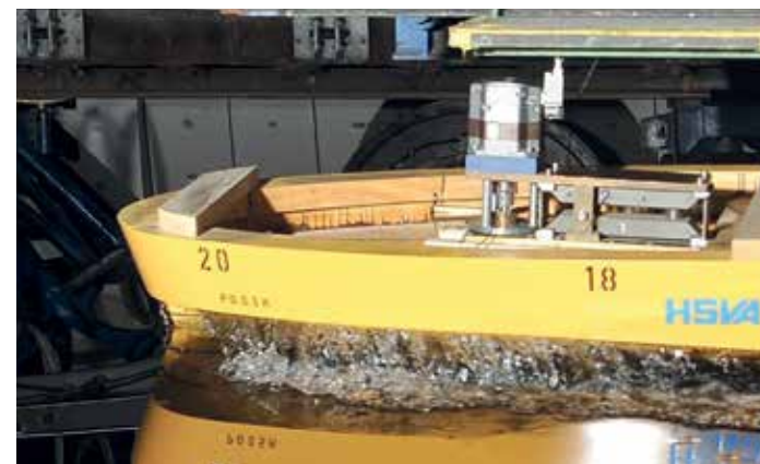
Figure 3: Bow wave of a double ended ferry in the towing tank
