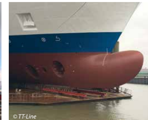
Figure 3: Fitting the optimised bulb to the bow of “Peter Pan”
