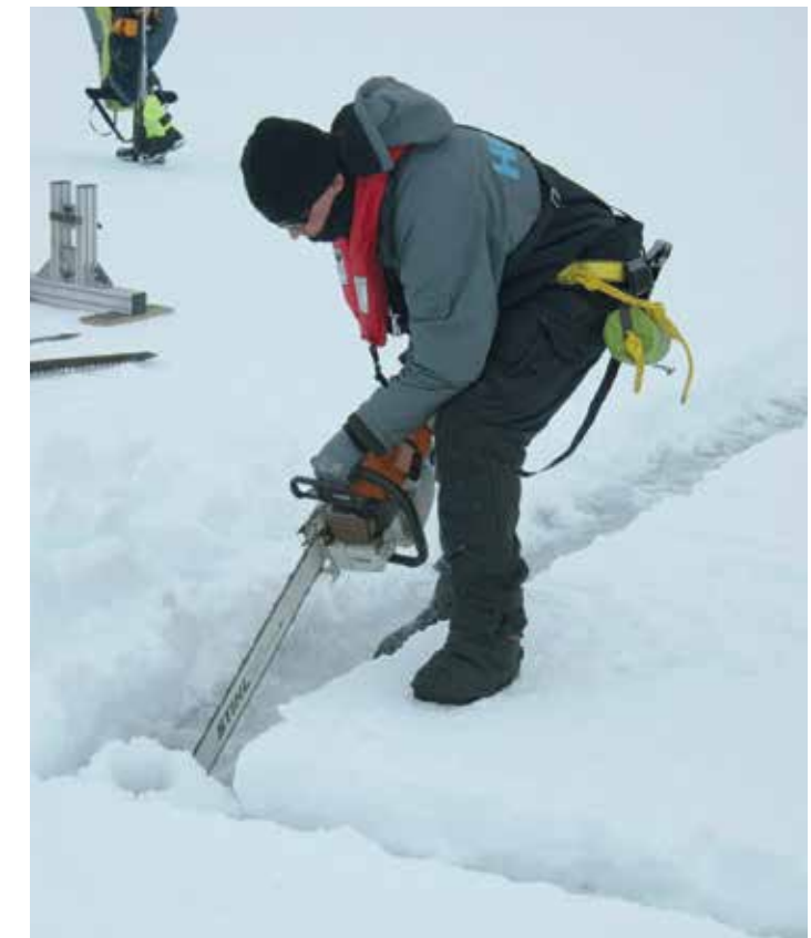
Figure 3: Full cantilever beam test for determination of ice flexural strength
