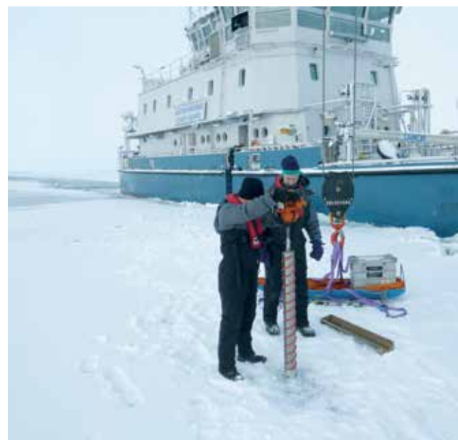
Figure 2: Drill hole measurement for ice thickness measurement (above), coring in ice to determine density, temperature, and salinity (right)
