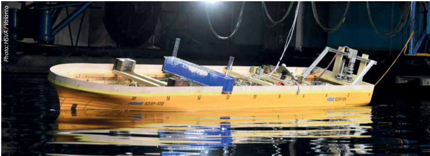
Figure 1: HERM test with a container vessel equipped with FLUME® anti-roll tank
