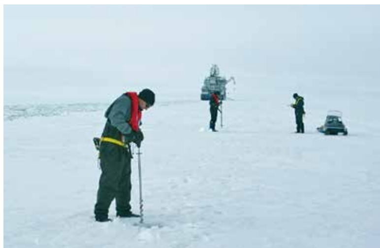
Figure 2: Drill hole measurement for ice thickness measurement (above), coring in ice to determine density, temperature, and salinity (right)
