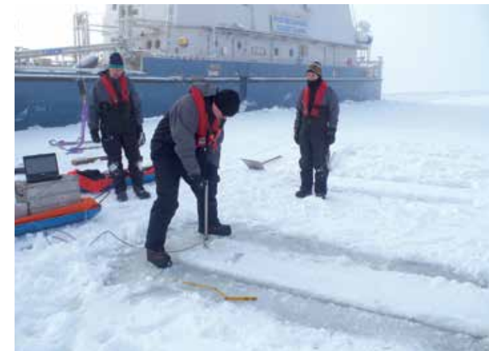
Figure 3: Full cantilever beam test for determination of ice flexural strength
