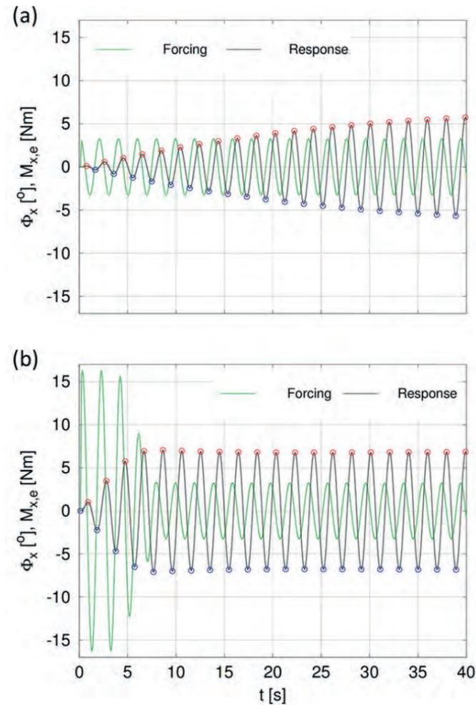
Figure 2: Excitation of roll motion (HERM) of the HCS bare hull (scale 1:52) at zero speed and an excitation moment amplitude of 3.25 Nm (a) without and (b) with the Artificial Induced Damping (AID) technique using an AID moment of 9.75 Nm
