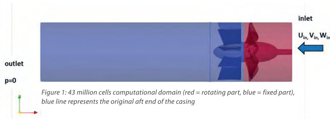
Figure 1: 43 million cells computational domain (red = rotating part, blue = fixed part), blue line represents the original aft end of the casing
