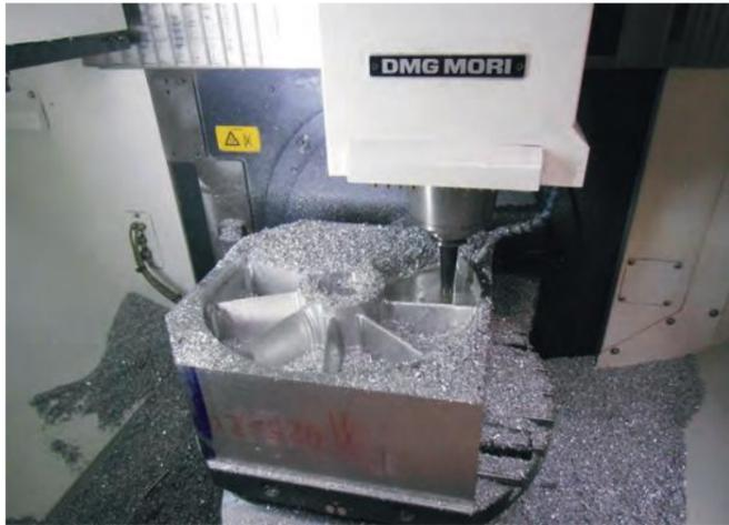
Figure 3: Milling process of the  $D = 410$  mm stator model
