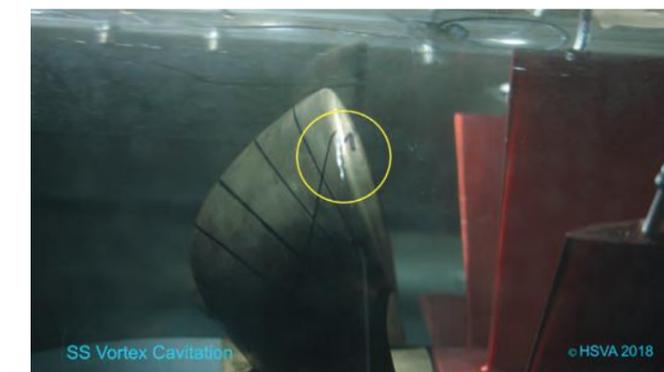
Figure 5: Back tip vortex cavitation occurring just under extreme overload conditions
