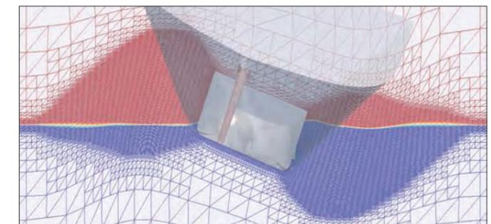
Figure 1: Cross cut through the CFD mesh highlighting the mesh deformation around the rolling ship hull. Colors show the location of the free surface between water (blue) and air (red)
