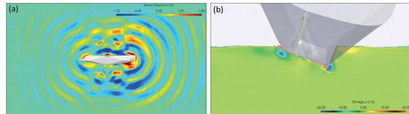
Figure 4: Roll motion of the HCS hull with 0.8-m bilge keels at zero speed. (a) Wave field looking from below, (b) axial vorticity in the mid-ship cross section
