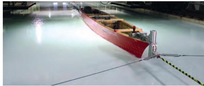
Figure 2: Resistance test in modelled level ice
