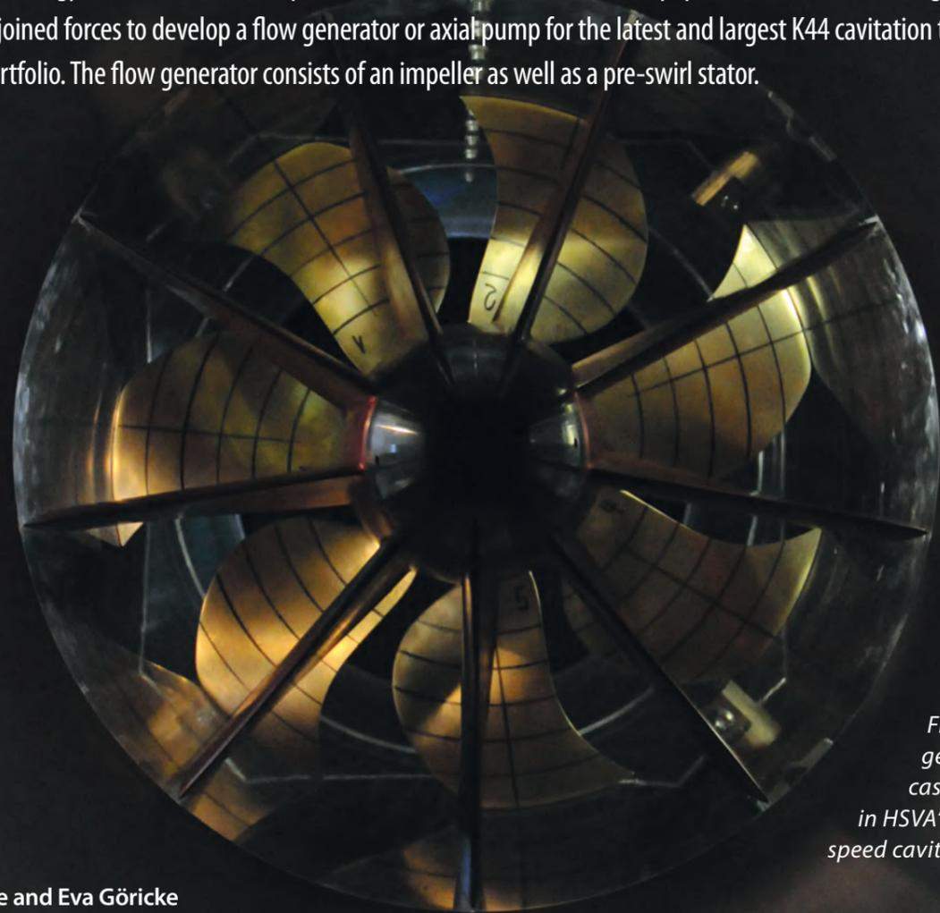
Figure 4: Flow generator and casing installed in HSVA's large high-speed cavitation tunnel
