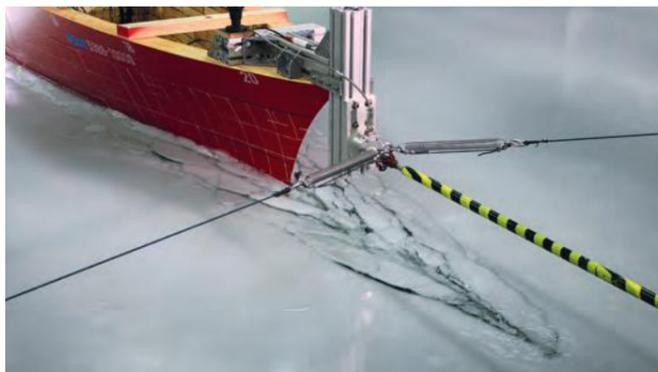
Figure 3: Breaking pattern of ship models bow taken at the end of the test run
