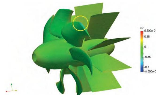
Figure 2: Surface pressure coefficient  $c_p$  and trace of limiting streamlines revealed from CFD
