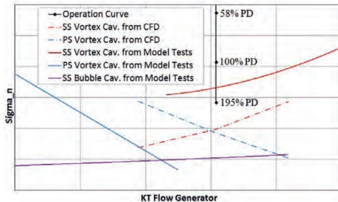
Figure 6: Cavitation diagram indicates absence of cavitation far beyond maximum power
