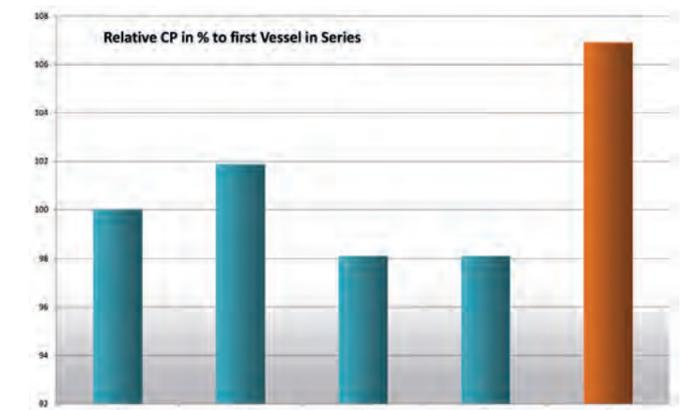
Figure 3: Relative deviation of power demand amongst 5 identical container vessels
