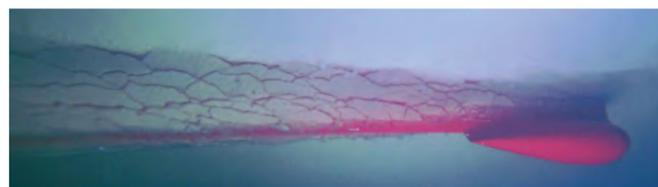
Figure 4: Underwater view of ship model being towed through level ice
