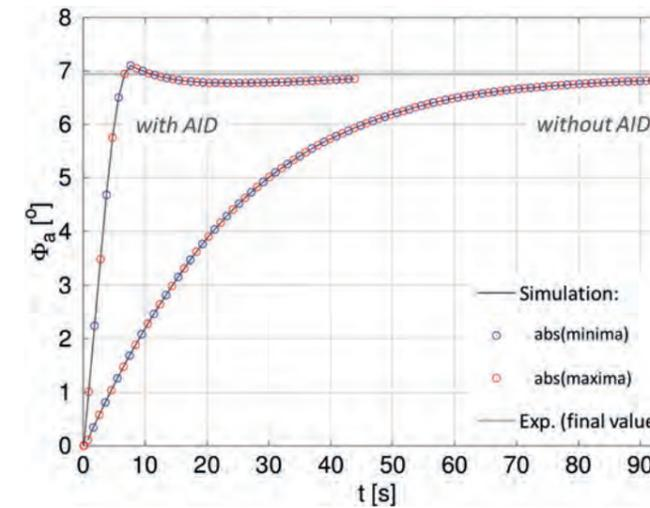
Figure 3: Evolution of the roll amplitude for the HCS bare hull at zero speed under moment excitation without and with the AID technique
