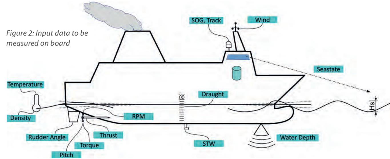
Figure 2: Input data to be measured on board
