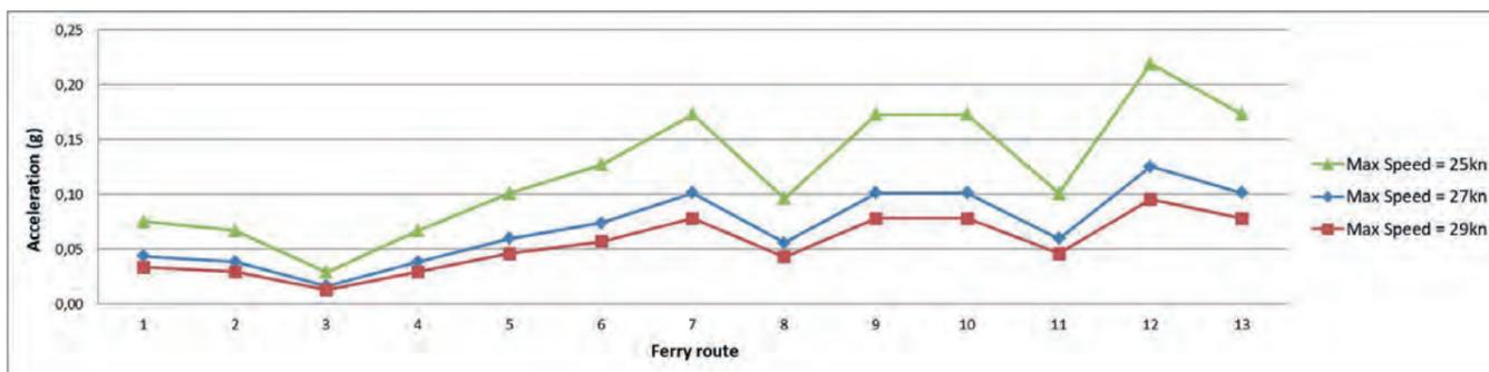
Figure 2: Required acceleration profile for different maximum speeds and pre-specified travel plan
