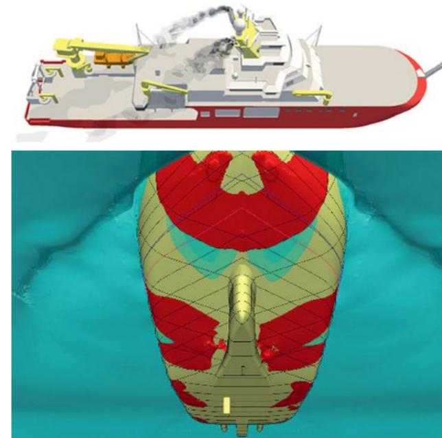
Figure 3: Exhaust gas dispersion simulation (top) and paint flow simulation (bottom)
