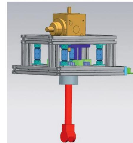
Figure 1: HSVA's construction of the pod scale
