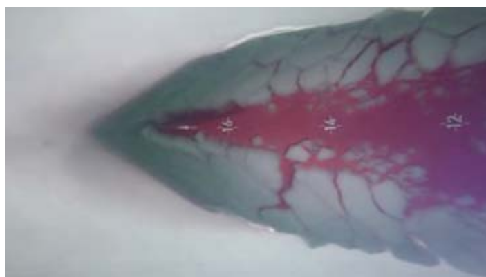
Figure 1: Investigation of ice flow along the hull to determine the influence of bow geometry
