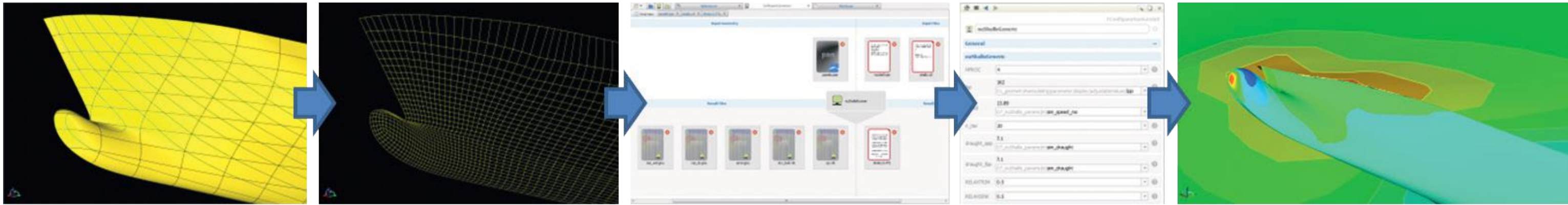
Figure 1: Hull form -&gt; Panelisation -&gt; Case setup -&gt; Computation -&gt; Result visualisation
