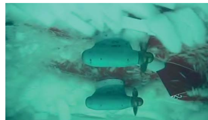
Figure 4: Ice flow into podded drives of an icebreaking supply vessel
