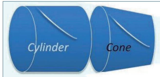
Figure 1: Two reference planes for a profile section orientation, left global cylindrical and right local cone
