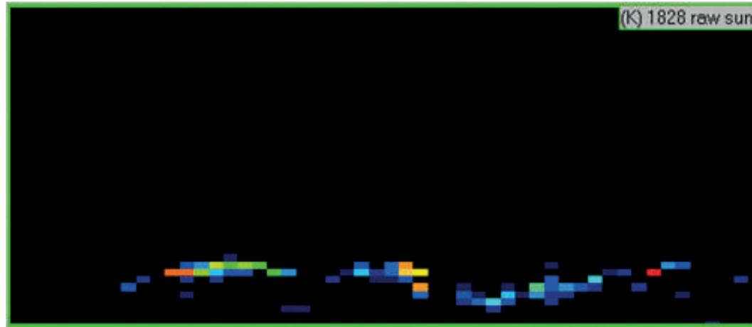
Figure 4: Snapshot from tactile sensor measurement showing the local ice pressure over the whole ice-structure interaction area for a cylinder with 200 mm diameter in new model ice
