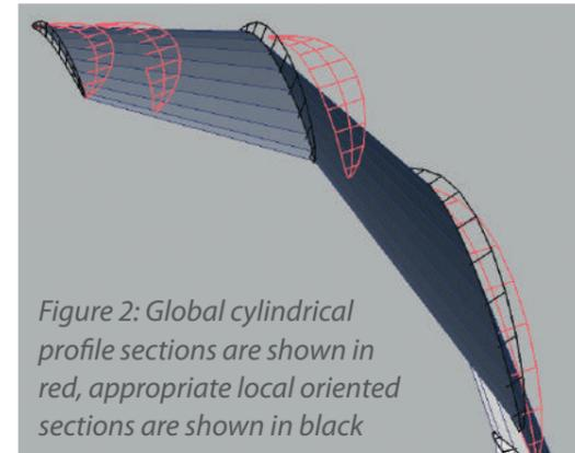
Figure 2: Global cylindrical profile sections are shown in red, appropriate local oriented sections are shown in black
