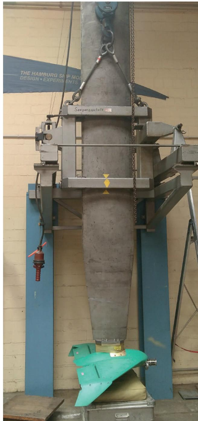
Figure 3: Depressor mounted at the „R39“ deep towing device – ready for installation on the towing carriage
