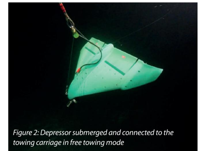
Figure 2: Depressor submerged and connected to the towing carriage in free towing mode
