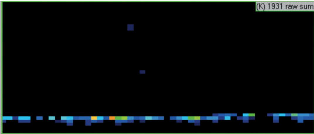
Figure 2: Snapshot from tactile sensor measurement showing the local ice pressure over the whole ice-structure interaction area for a cylinder with 200 mm diameter in current model ice
