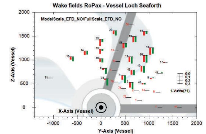
Figure 4: Comparison of the local nominal wake fraction, measured in HYKAT (red) and in full scale (green). (Source: University of Rostock)
