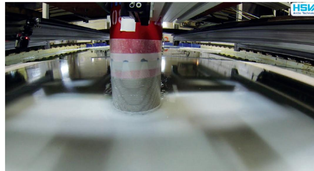
Figure 3: Cylindrical model crushing through current model ice (left) and new model ice (right) during FATICE tests
