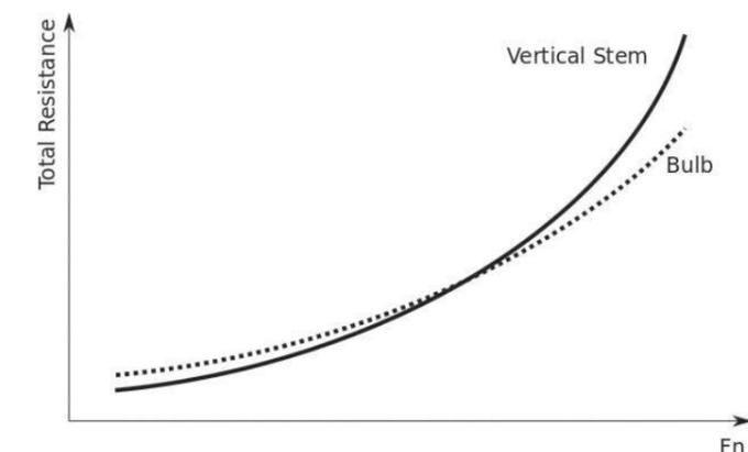
Figure 2: Generic resistance curves showing the fundamental effect observed for the different bow concepts
