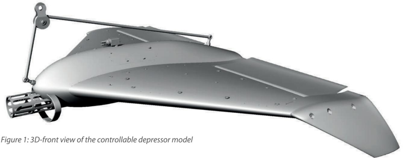
Figure 1: 3D-front view of the controllable depressor model
