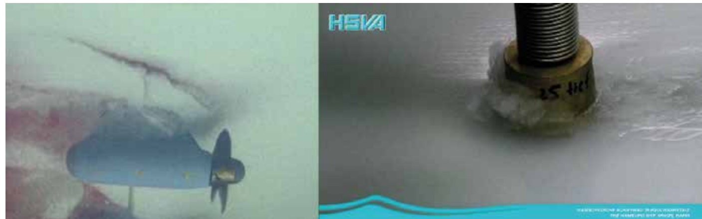
Figure 2: Ice crushing at azimuth housing (left), indentation test to determine the model ice crushing strength (right)
