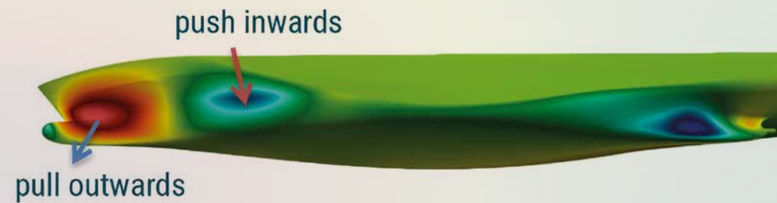
Figure 1: Result of a single adjoint computation at the KCS container ship showing the sensitivity map in y-direction indicating where to modify the hull form to get better hull form resistance.
