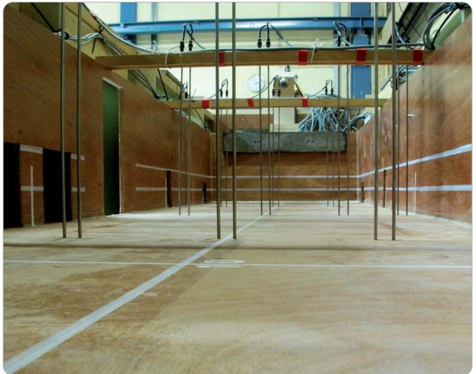
Fig. 2: A view of the vehicle deck during the outfitting of the model. In full scale the deck is about 44 m long. The arrays of the wave probes cross the otherwise open deck. The large black opening on the left side wall is the modeled collision damage by another ship bow.
