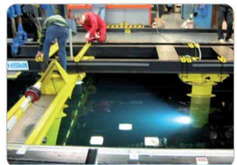
Fig. 4: Towing carriage installation
