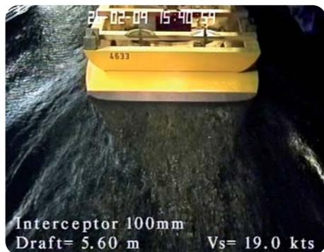
Fig. 3: Transom flow off the ducktail with and without interceptor
