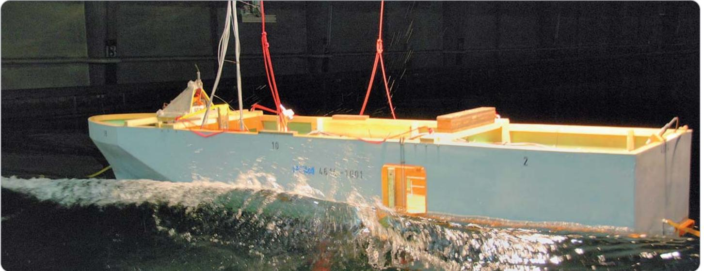
Fig. 1: A ship model in an early phase of a damage stability test in waves in the HSVA towing tank. The photograph shows a breaking wave just before it hits the damaged ship side and pushes considerable amount of water through the damage opening mainly on to the vehicle deck.
