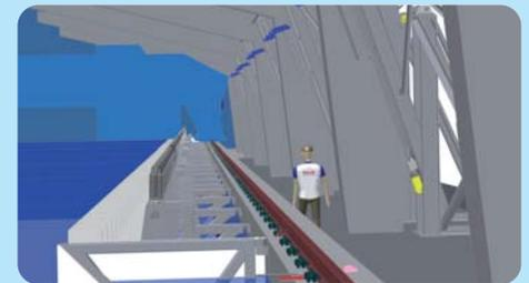
Fig. 1: Impression of the new side wave generator in the Large Towing Tank
