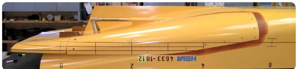
Fig. 2: The model of the 'after conversion' Hammerodde under construction in HSVA's model workshop
