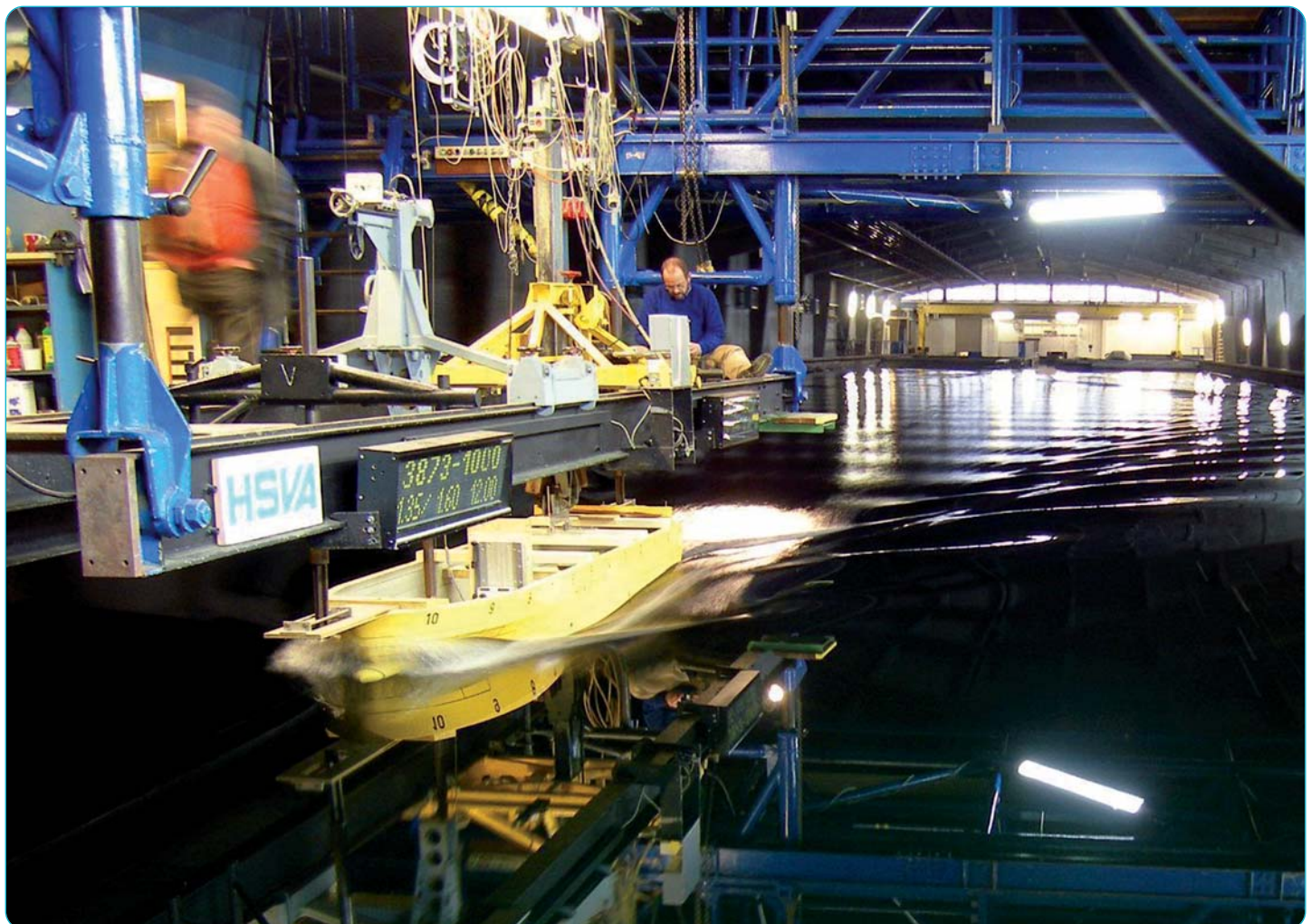
Model ferry fitted with bulbous bow in HSVA's large towing tank
