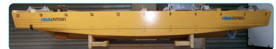
Fig. 2: View of the appended Model (without VSP) for the resistance test
