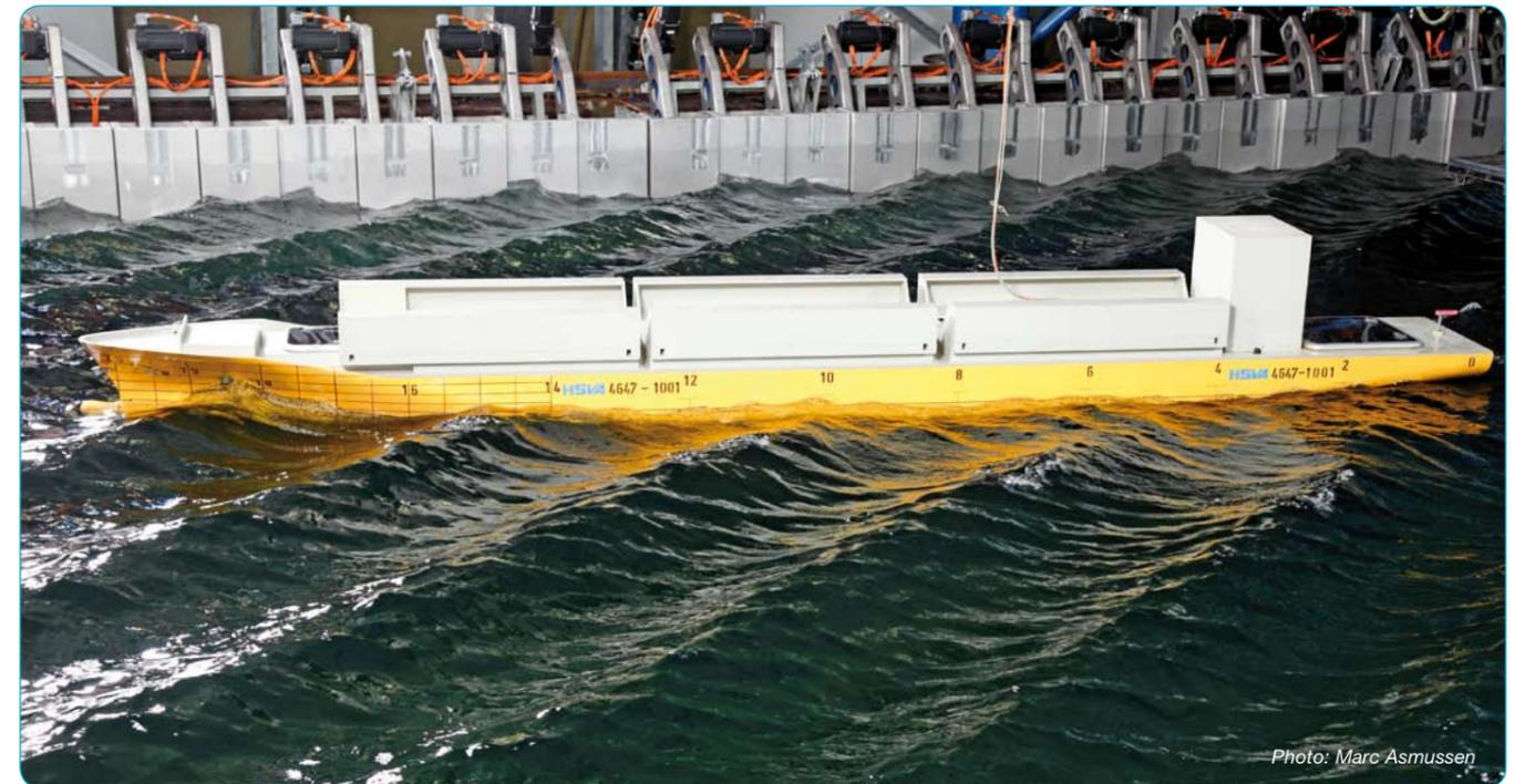
Fig. 1: A container ship model advancing in short oblique waves generated by the new Side Wave Generator in HSVA’s large towing tank
