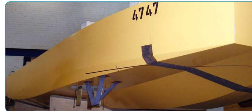
Fig. 1: VSP and protection girder arranged on the starboard bow
