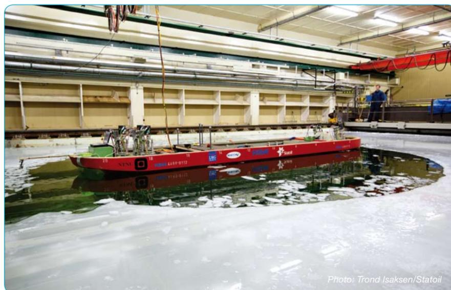
Fig. 1: Drill ship model has performed a full turn in level ice solely controlled by DP
