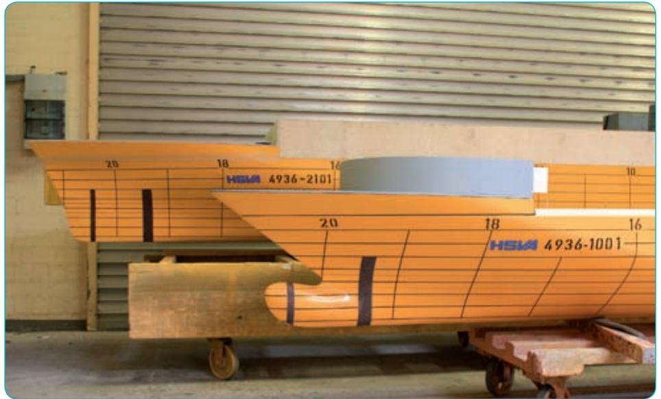
Fig. 2: Two different bow forms of the hull were tested and compared.
