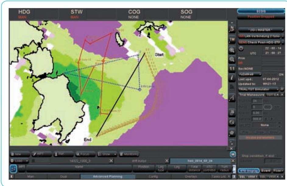
Fig. 6: Screenshot of ECDIS System on board R/V Lance showing ice thickness chart (background colors), optimized route (brown), helicopter track (blue) and drift buoy track (red)
