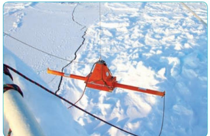
Fig. 3: EM-31 mounted at R/V Lance bow
