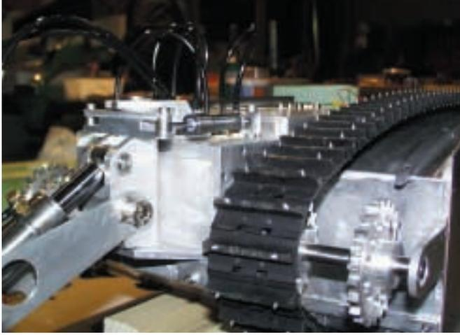
Model of front unit with link arm and hydraulic ram
