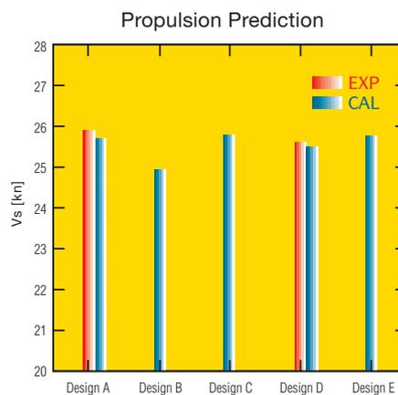
Fig. 1: Attained ship speed of the 5 propeller designs
