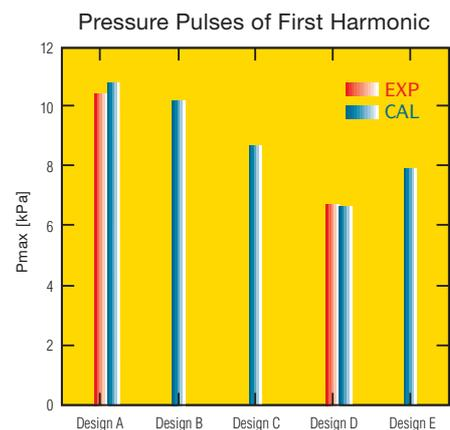
Fig. 2: Pressure pulses of the 5 propeller designs
