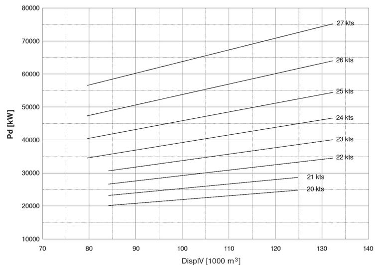
Required power at the propeller for very large container ships (6000 TEU to 9000 TEU)
