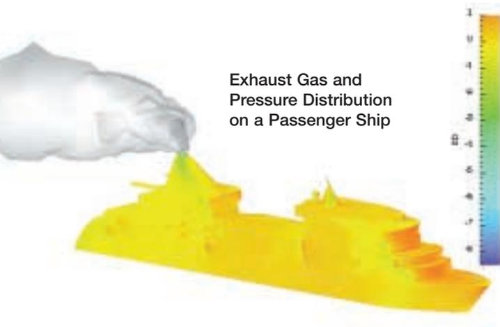
Exhaust Gas and Pressure Distribution on a Passenger Ship
