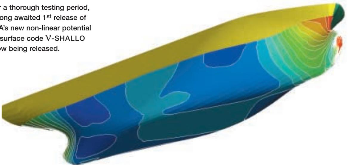
This all new CFD code will boost performance during design analysis and optimisation. The programme has been developed using latest singularity as well as numerical techniques. Advanced programming concepts make it an “easy to use” window oriented application that will integrate smoothly into a variety of design environments.
