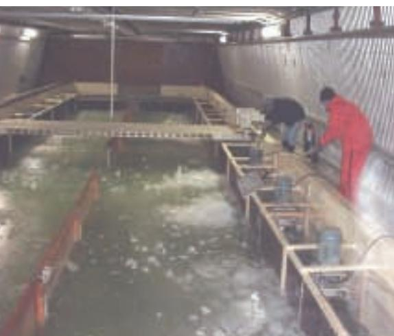
Fig. 2 Propeller arrangement in the recirculating flume
