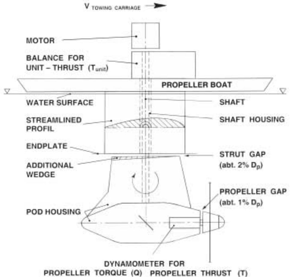
Fig. 1 Pod open water test setup
