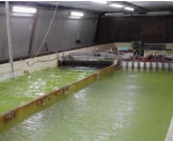
Fig. 1 Twin wave tank and two separately operated paddles
