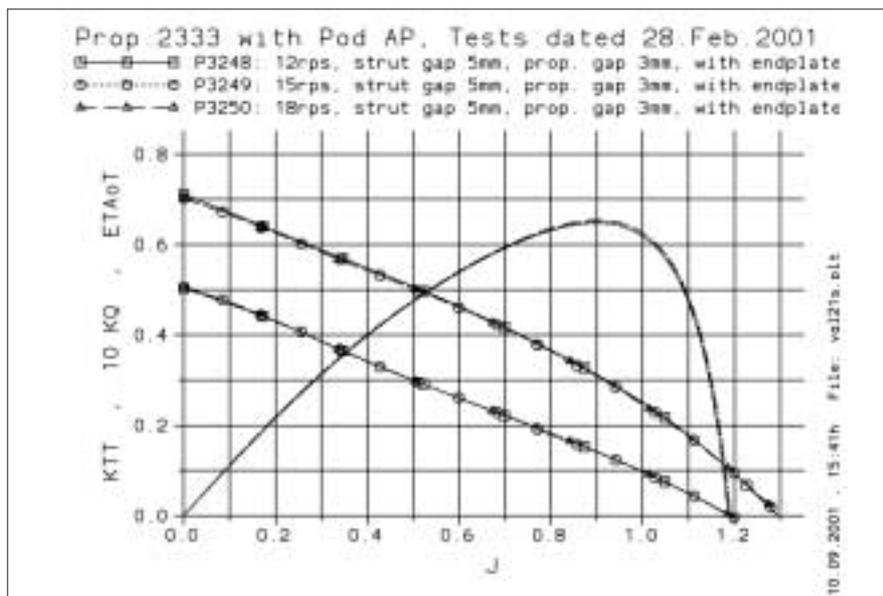
Fig. 2 Open water characteristics of a pod unit for different propeller speeds (based on measured unit thrust)
