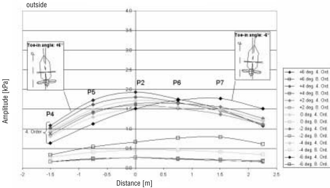
Fig. 3 Distribution of Pressure Fluctuations
