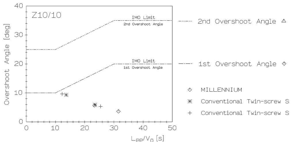
Fig. 4 IMO Criteria regarding overshoot angles at 10°/10° Zigzag Manoeuvre
