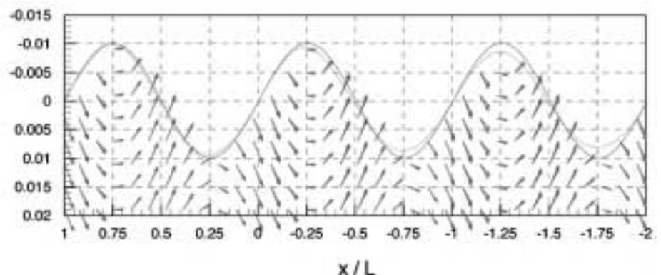
Simulations of the Series 60 ship moving straight ahead in harmonic head waves at  $F_n=0.316$  show that the pronounced wave system of the ship is only moderately distorted by the long, small oncoming waves considered in this case, Fig. 3 and 4.
