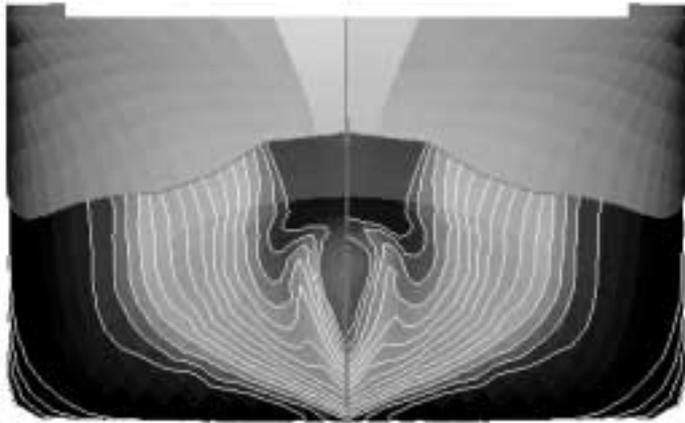
Pressure distribution for original (left) and modified (right) hullform
