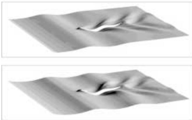
Fig. 4 Two snapshots of the simulation of the flow around the Series 60 ship in head waves
