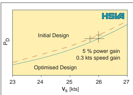
C/V - 5.618 TEU, comparison of speed-power curves initial design with optimized design
