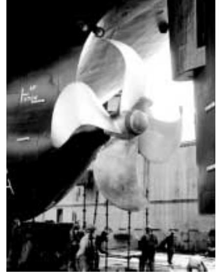
The KAPPEL propeller blade geometry based on the principle of non-planar lifting surfaces
