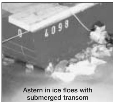
Fig. 3 Performance tests in ice floes of 0.4 m ice thickness, astern with submerged and emerged transom
