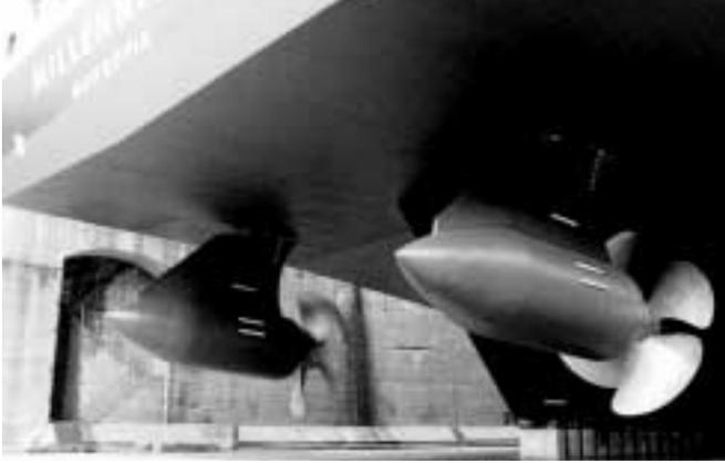
Fig. 1 Full Scale POD Arrangement
