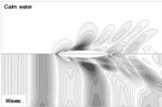
Fig. 3 Computed wave patterns of Series 60 ship in calm water and in head waves
