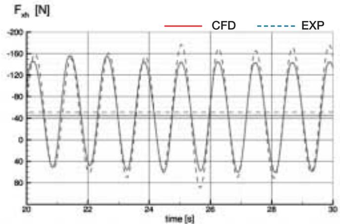
Fig. 5 Computed and measured longitudinal force at a container ship model in head waves
