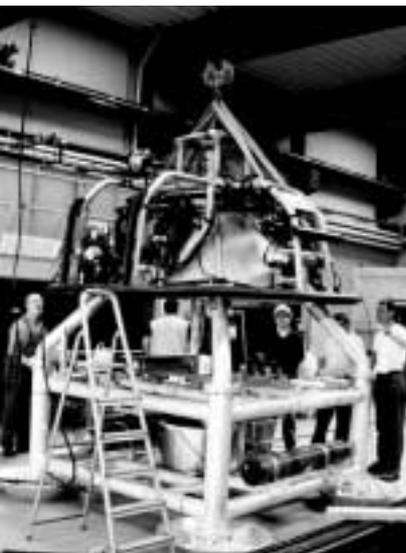
The recovery vehicle MODUS is docked to the ground station (GS)
