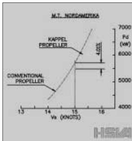
The observed cavitation phenomena showed an improvement compared with the conventional propeller, and consequently excitation forces arising from the action of the propeller were also improved.
