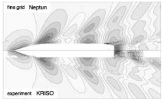
**Fig. 1** Computed and measured wave patterns of the KCS at Froude number  $F_n=0.26$ . Blue areas denote crests and grey areas troughs.
