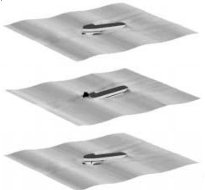
Fig. 7 Simulation of the motions of a container ship in head waves
