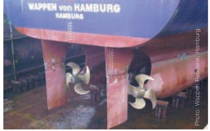
Fig. 2 SCOT 8000 "Wappen von Hamburg" ready for service (SCOT Safety Chemical Oil Tanker, 8000 DWT)
