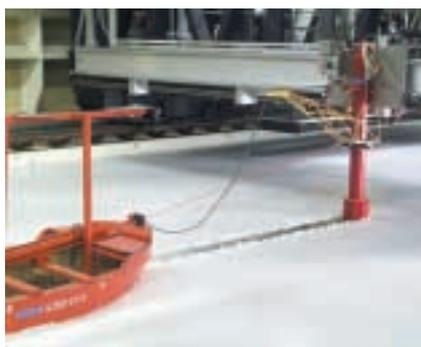
**Fig. 4 Straight ice drift – managed ice**
