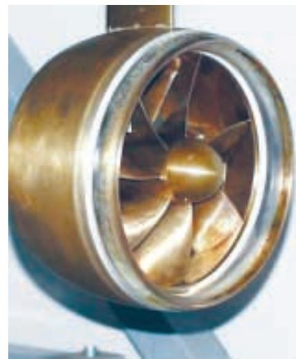
**Fig. 2 Scale model RDP**
