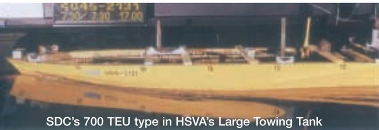
SDC's 700 TEU type in HSVA's Large Towing Tank
