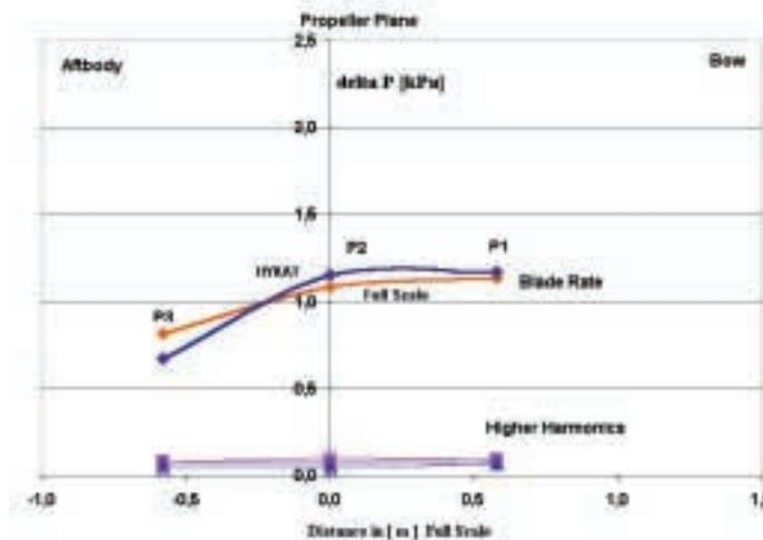
Fig. 3 Comparison of Pressure Fluctuation Data Full scale / HYKAT
