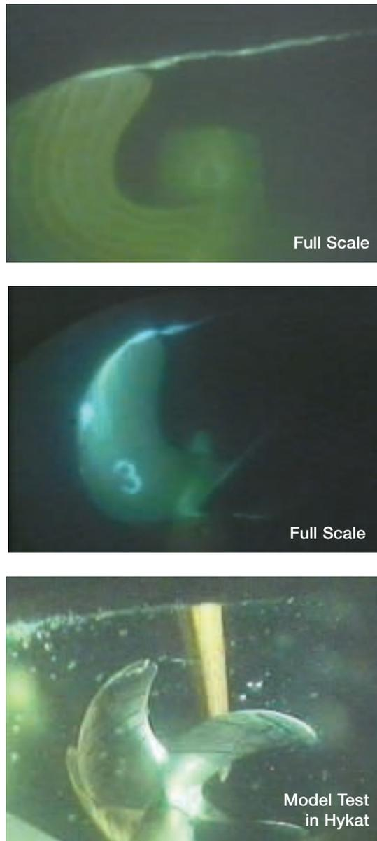
Fig. 2 Comparison of Cavitation Phenomena Full Scale / HYKAT
