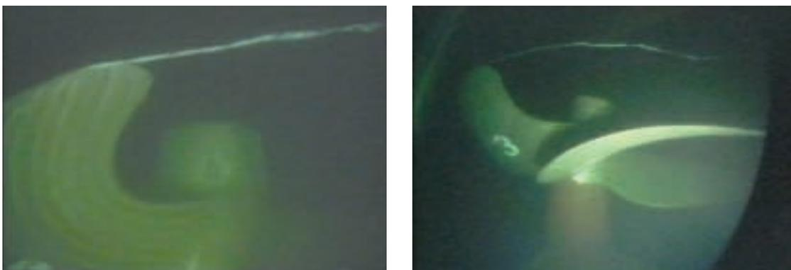
Fig. 1 Full Scale Tip Vortex Cavitation 100% MCR
