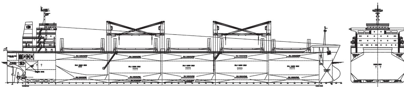
General Arrangement of the 57,300 DWT Super-Handymax Bulk Carrier
