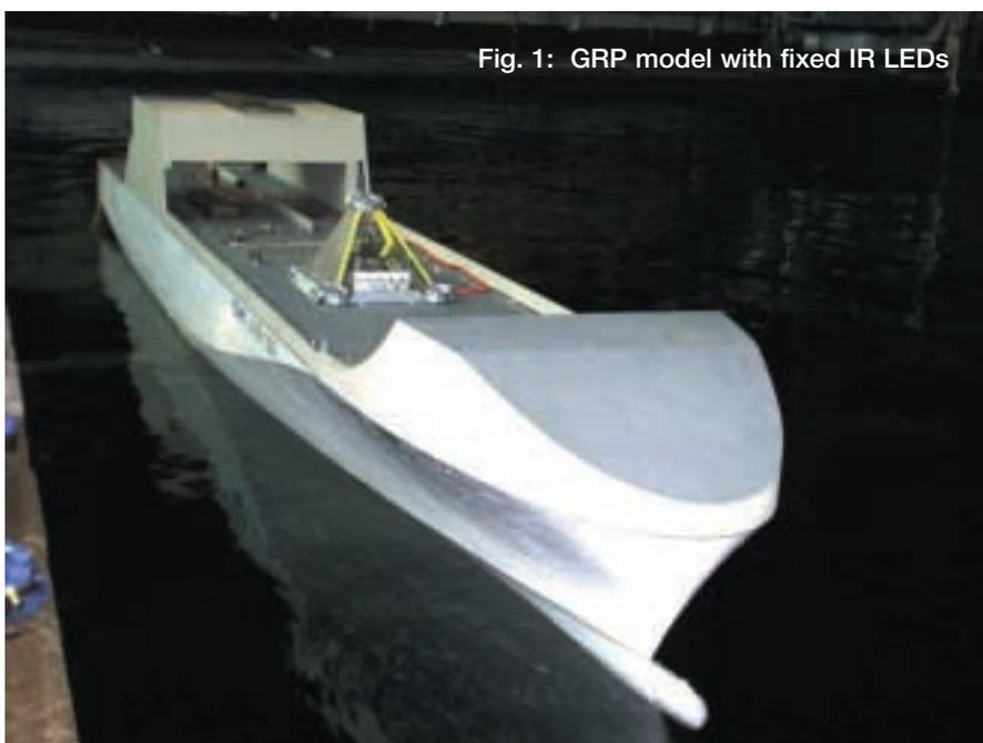
Fig. 1: GRP model with fixed IR LEDs
