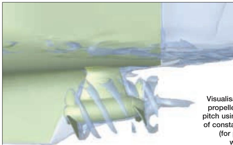
Fig. 3: Visualisation of the propeller slipstream pitch using surfaces of constant vorticity (for pod variant without fins)
