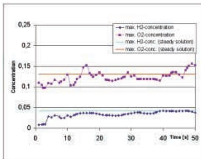
Development of the maximum hydrogen and oxygen concentration as function of time. The highest gas concentration is usually reached shortly after the start of the recharging.
