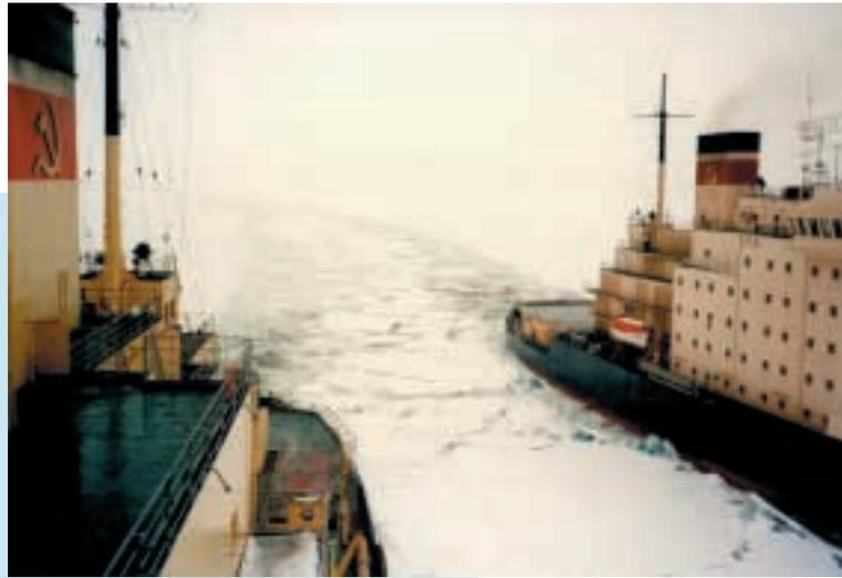
**Fig. 4** Preparation of a wide ice channel with the help of two icebreakers in model and full scale
