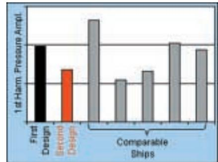
Fig. 2 Hull Pressure Pulses CV 4050
