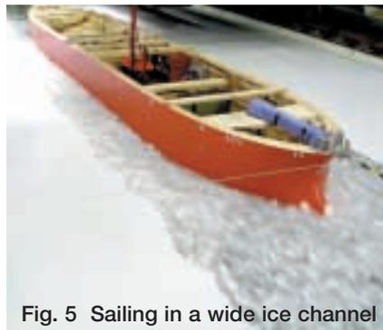
**Fig. 5** Sailing in a wide ice channel
