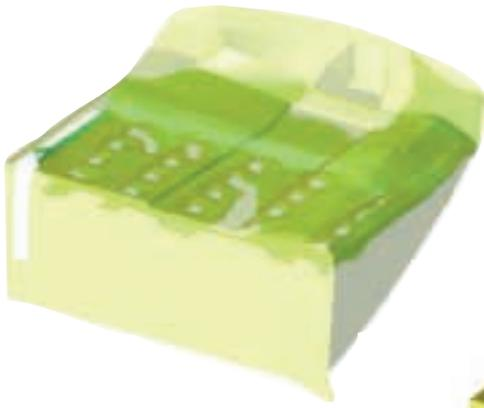
Computed isosurface of one percent hydrogen concentration shown under the semitransparent bonnet.
