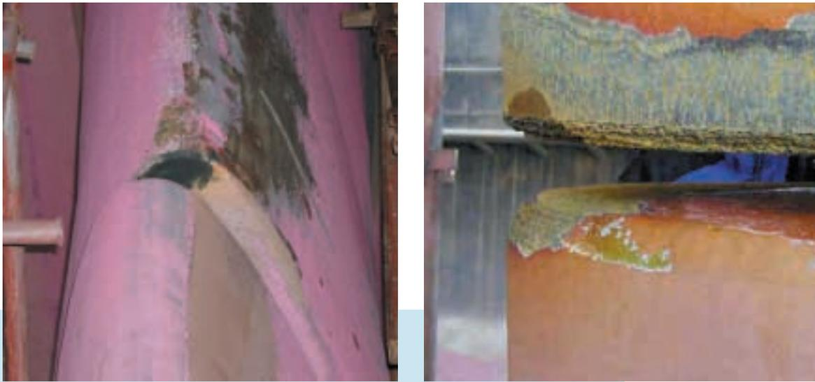
Fig. 2 Rudder Damages
