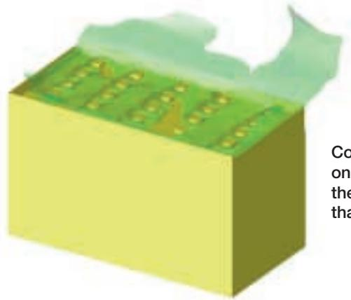
Computed isosurface of hydrogen on the battery. Above the isosurface the hydrogen concentration is higher than one percent, below it is lower.
