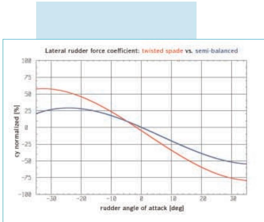
Fig. 3 Comparison of the Lateral Rudder Force Coefficients
