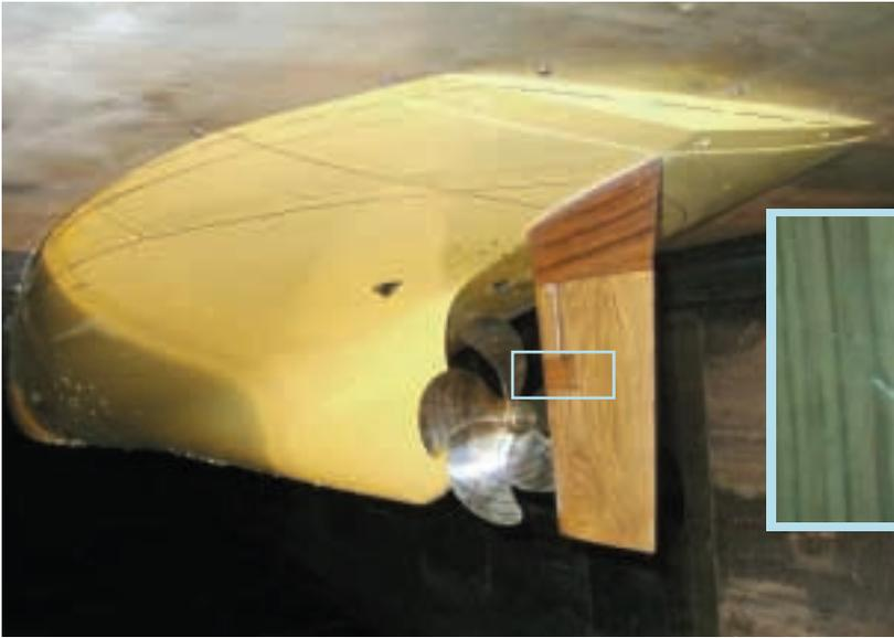
**Fig. 2 Rudder Cavitation Test with the Entire Ship Model in HYKAT**
