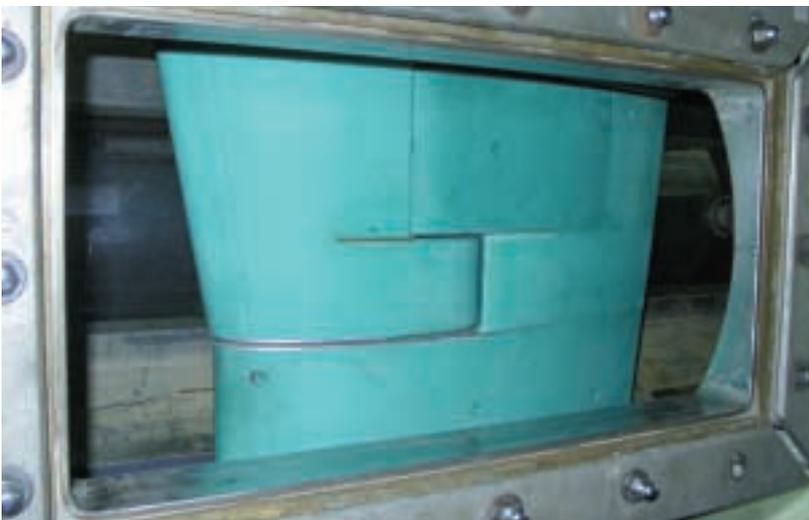
**Fig. 3 Increase of Rudder Cavitation Tests carried out at HSVA**
