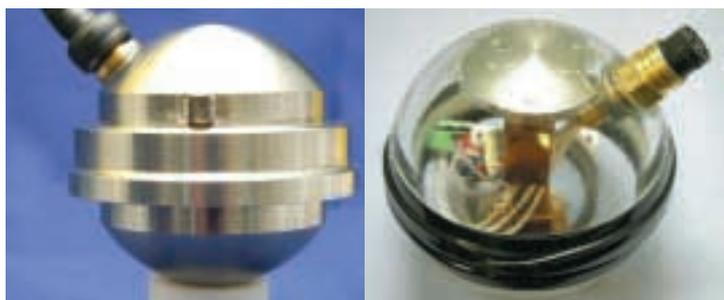
**Fig 4: The 12cm diameter iron ball and glass ball sensors calibrated at the HSVA ice tank**
