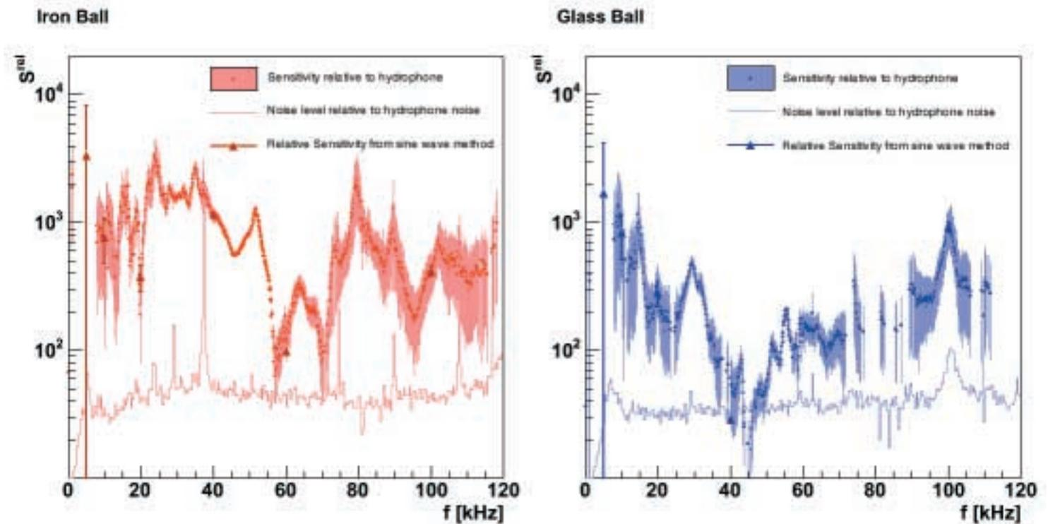
Fig. 5: Relative sensitivity vs. frequency for the iron ball sensor and the glass ball sensor
