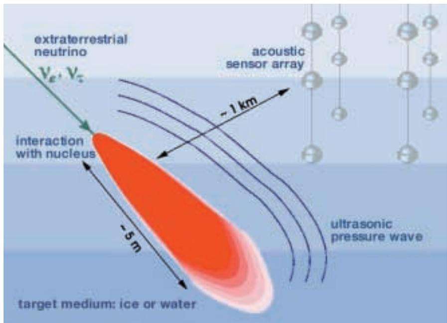
transmitters. These are usually build on the basis of piezo ceramics, which are also used in commercial hydrophones. When applying a compressive force to the ceramic, an electrical signal is produced, which can be amplified and recorded. Due to the pressure of up to 500 bars which will develop in the deployment in the ice, the use of pressure housings, either of glass or metal is necessary to protect the electronic circuits (see Fig. 4).
