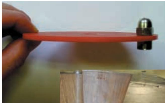
Fig. 2: Discs with Eccentric Mass(es) for Calibration
