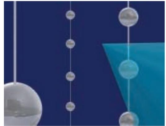
Fig. 1: Light is generated in a neutrino interaction in the ice and registered by light sensors in pressure balls
