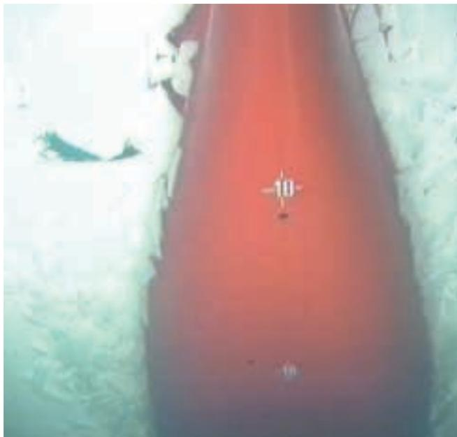
**Fig. 2: Under Ice Observation during an Ice Model Test of a LNG Carrier (view from underneath)**
