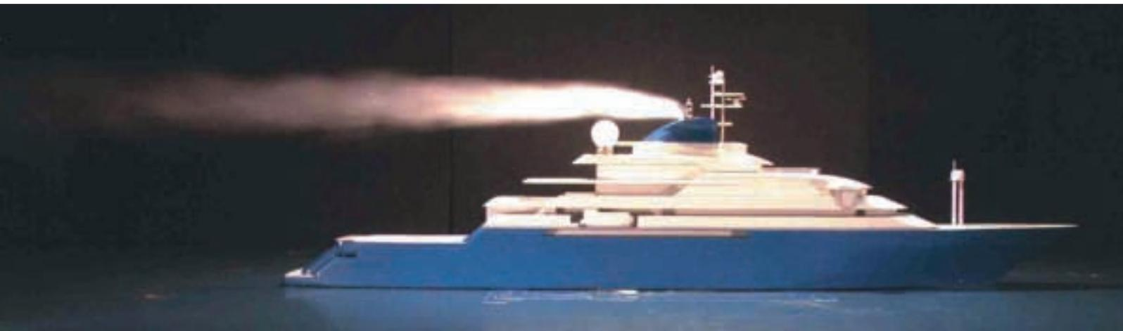
**Fig. 2 OCTOPUS model in the wind tunnel**
