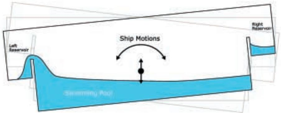
Fig. 2: Generic sketch of pool cross-section, ship motions and expected overflow
