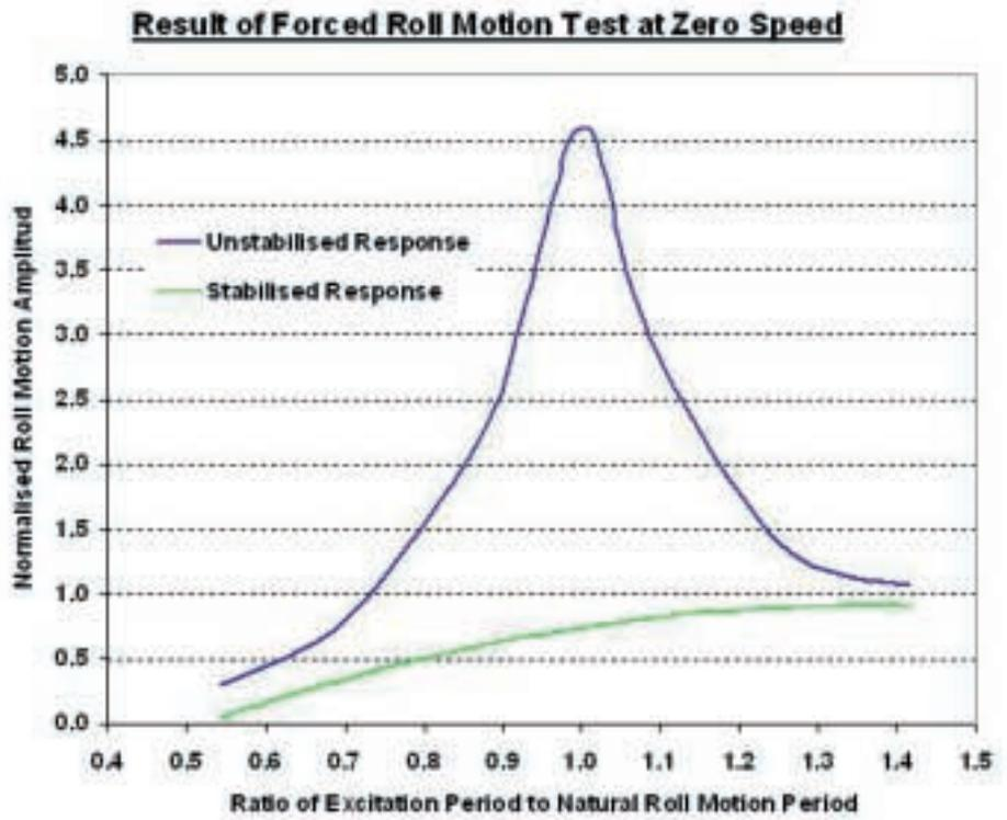
Fig 2: Harmonic roll motion response with active and passive roll damping arrangement
