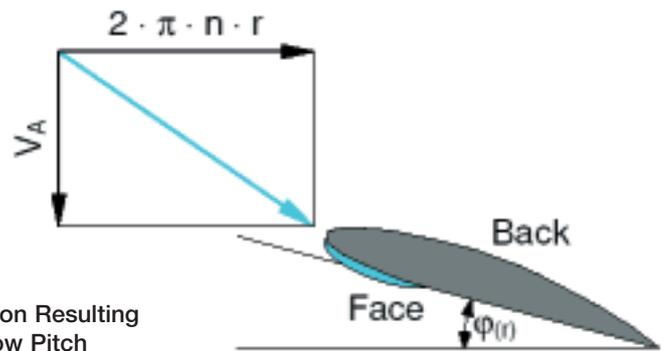
Fig 3: Face Cavitation Resulting from a too Low Pitch
