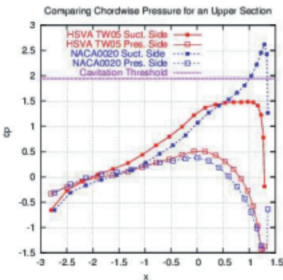
Fig. 3: Improved pressure at rudder nose
