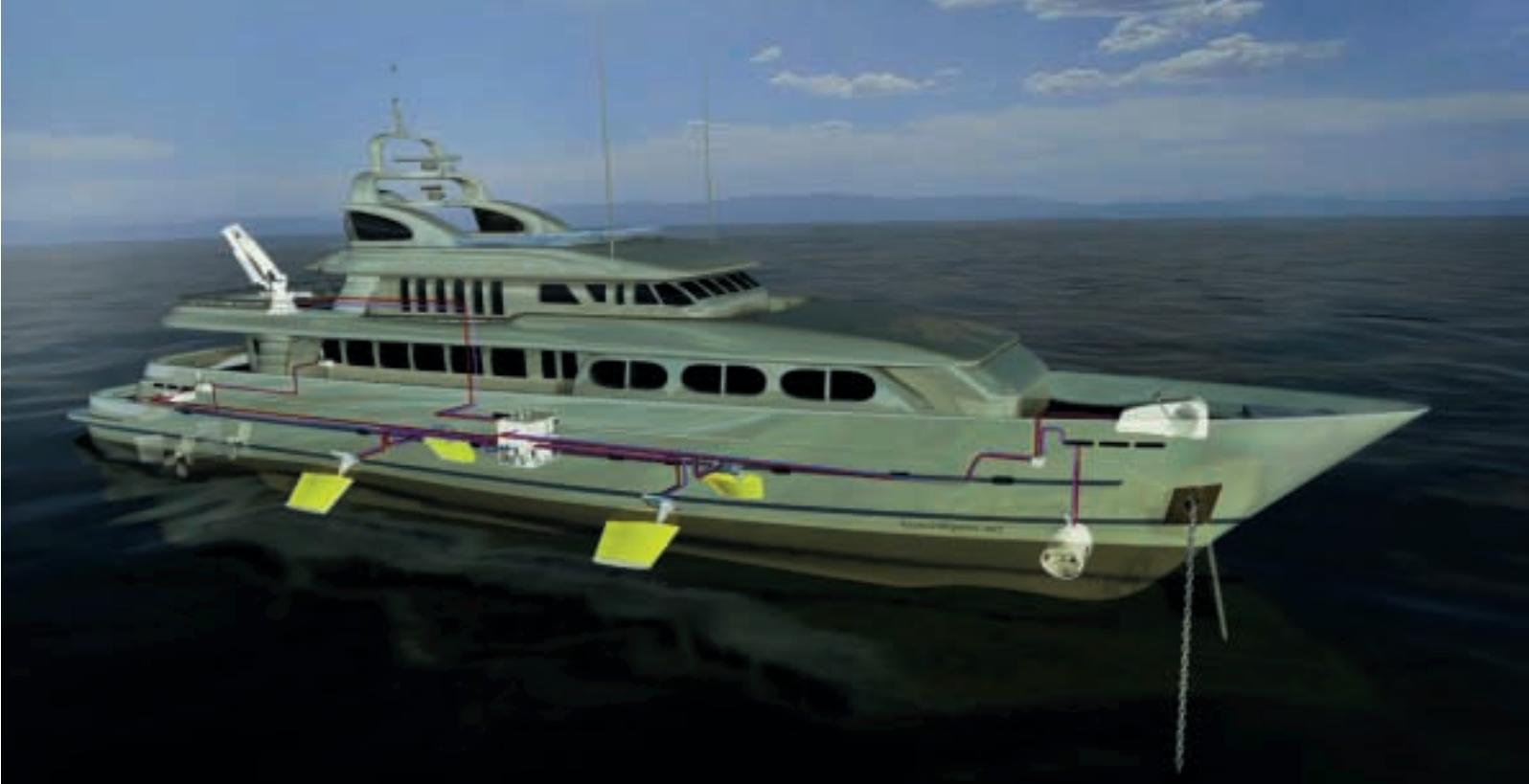
Fig 1: Artist's impression of a motor yacht with two sets of stabilising fins.
