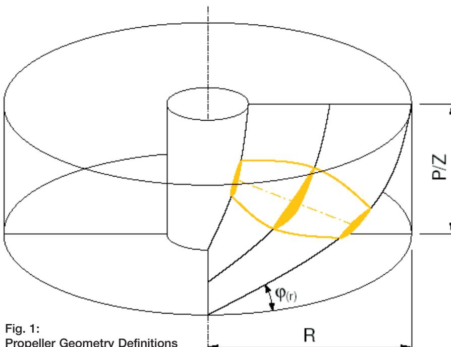
Fig. 1: Propeller Geometry Definitions
