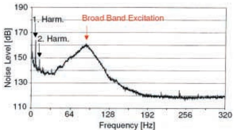
Fig 4: Broad Band Excitation of a Passenger Vessel at Low Speed
