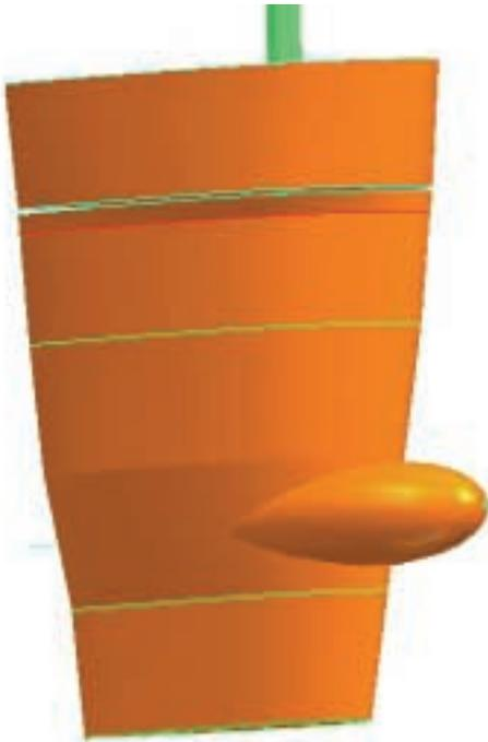
Fig. 1: HSVA TW05 rudder (with bulb)
