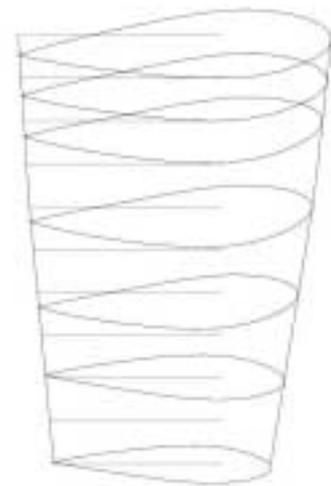
Fig. 2: Section geometry of HSVA TW05 visualized
