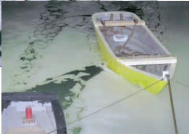
LNG-Carrier. The test program should also include ice-breaking tests at loaded draft in ice. But model tests are not only performed in order to analyse the required power and thrust, it is also very important to investigate the manoeuvrability of the projected LNG-Carriers in ice.
