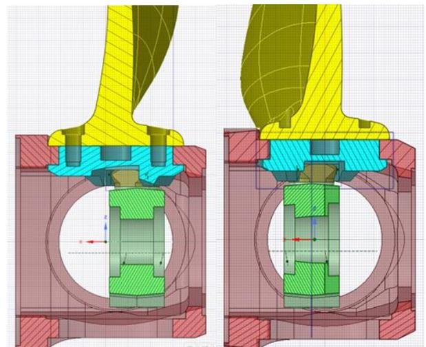
Depict: Propeller pitch mechanism geometry at forward and backward ship speed
