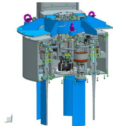
Depict: Section through VSP model propeller equipped to measure loads on blades and blade actuating gear
